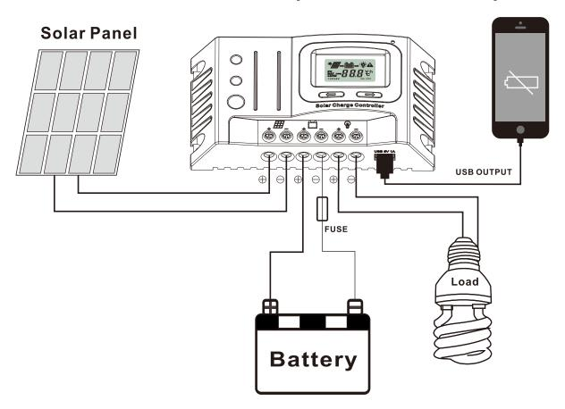
1) As figure, first connected the battery to controller correct poles. In order to avoid short circuit, please screw the cable of battery to the controller in advance, then connected to battery poles secondly. If your connection is correct, the LCD displaying will show battery
